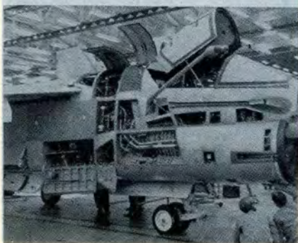
A-7A with access panels open. Work areas are readily accessible so that maintenance can be performed easily, right at working levels.
