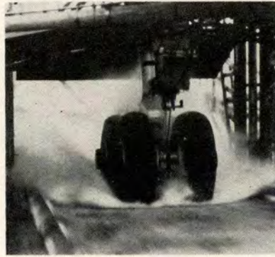
Front view of spray patterns at partial (left) and total hydroplaning speeds. Tire pressure: 5 lb/in 2 ; slush depth one inch. Photos were taken during tests at NASA Langley track.
